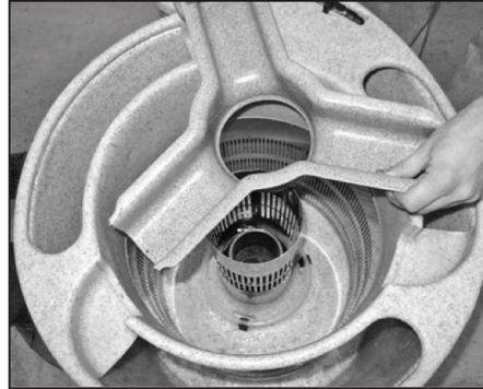
2. Remove the stainless steel perforated centre pipe by pulling gently.
