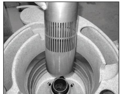
8. Refit the steel pipe with the perforations at the top, not at the bottom.
