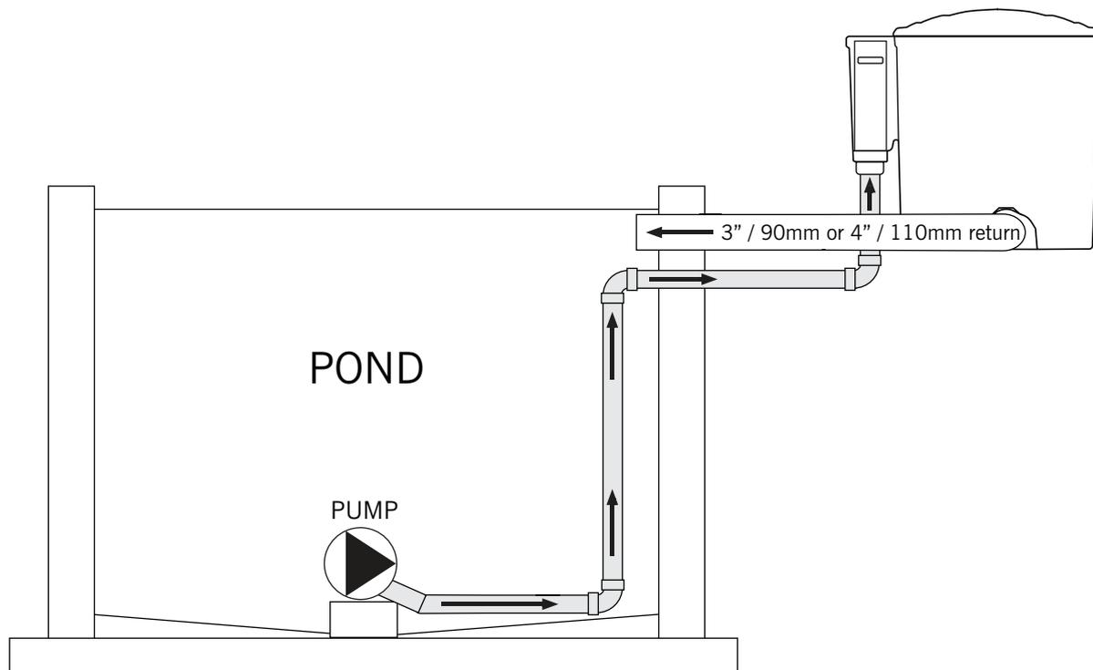
**PLEASE NOTE:** The pump must not be placed on the base of the pond, as failure in the pipework or connectors could lead to complete drainage of the pond. The pump should be raised at least 12" off the ground or high enough to leave sufficient water for the fish to survive, in the unlikely event that this occurs.
